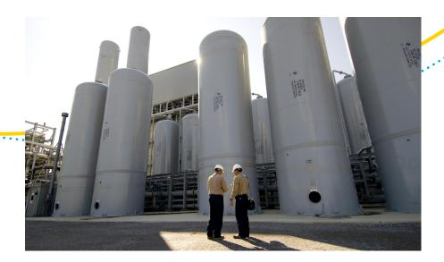
Air Products owns and operates more than 70 PSA systems worldwide for the purification of hydrogen.
