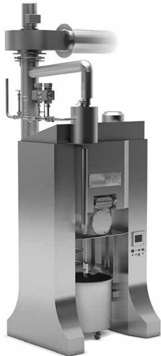
Mixer fitted with LIN-IS top injection technology
