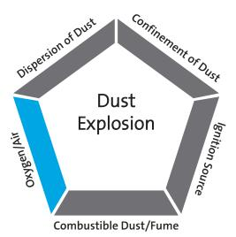
Unlike mechanical explosion control systems, using inert gas systems for combustible dust handling can prevent an explosion before it starts by removing the oxidant required for an explosion. Nitrogen inerting is a practical solution to help prevent the devastation to personnel and property that can result from combustible dust explosions.
