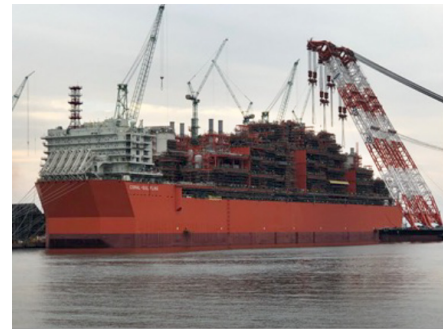
For the Floating LNG (FLNG) facility, ENI Coral South, the CWHE equipment was installed into modules at the shipyard utilizing Air Products' dual mixed refrigerant (AP-DMR™) LNG Process.
