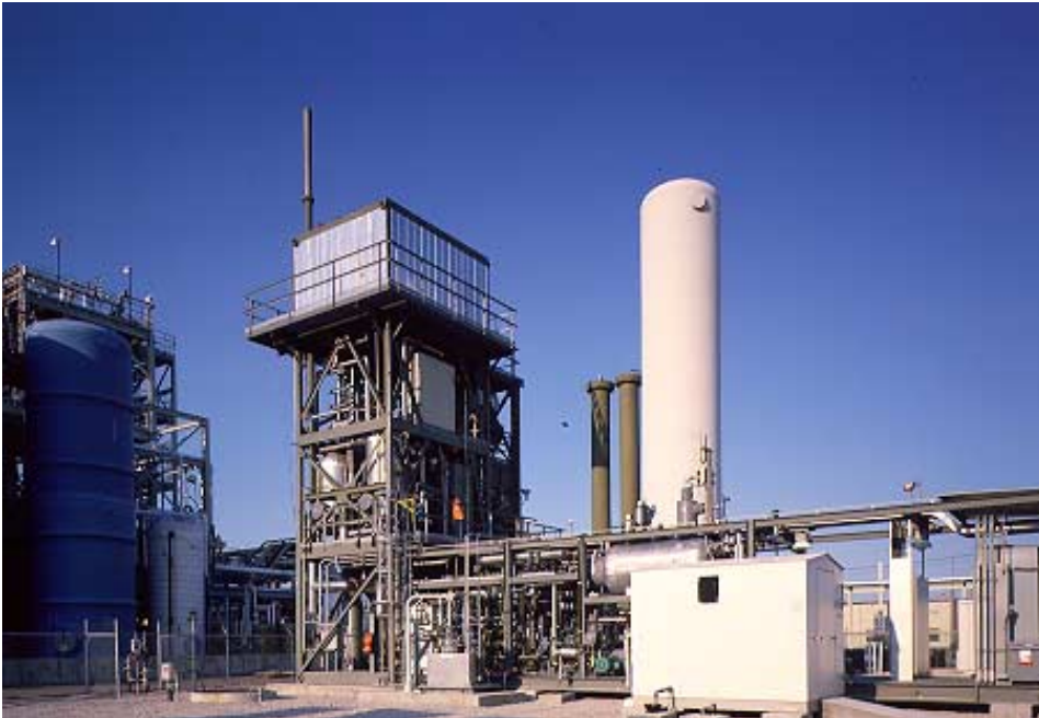
SMART H 2 plants provide significant savings in capital, maintenance and operating costs for facilities requiring hydrogen capacities above 0.5 million scfd.
